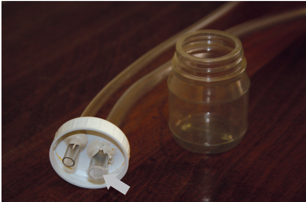
An aspirator used for collecting insects. Ensure that the gauze filter (arrow) is always in place.
